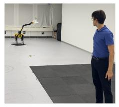
moving the camera in space-similar to how humans reposition their arms or heads to follow a moving object. This enhanced perceptual mobility is crucial for maintaining visibility of the ball, especially during fast, dynamic trajectories.
