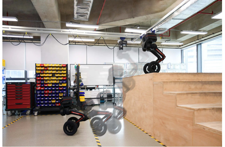
Figure 1: LIMX Dynamics TRON1 robot—a bipedal wheeled platform with 3 actuated joints and one wheel per leg (4 DoFs per leg total)
